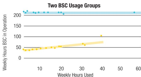
Figure 3: Results showing hours/week when users are working in BSCs (yellow) and hours BSC blowers were left operating regardless of active usage (blue). Average weekly use is 18 hours/week.\*
