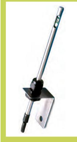
A **thermal or "hot-wire" anemometer** may also be used to independently measure airflow. Anemometers use a heated wire to measure airspeed, the more air crossing it, the more it's cooled, changing its electrical resistance. While these devices can trigger an audible or visual alarm for airflow specification deviation, they are limited to taking a reading at a single point in the airstream.
