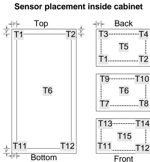
16 thermocouples were mounted inside the cabinet for temperature measurements. The locations of the TC sensors were the same for all ULTs except thermocouple 16 (T16). T16 was mounted within 1” of the temperature probe. Therefore the location of the T16 is dependent on where the temperature probe is. Some models were in the middle of the cabinet but some were at the bottom. Note: All shelves were taken out for all ULTs for performance testing.
