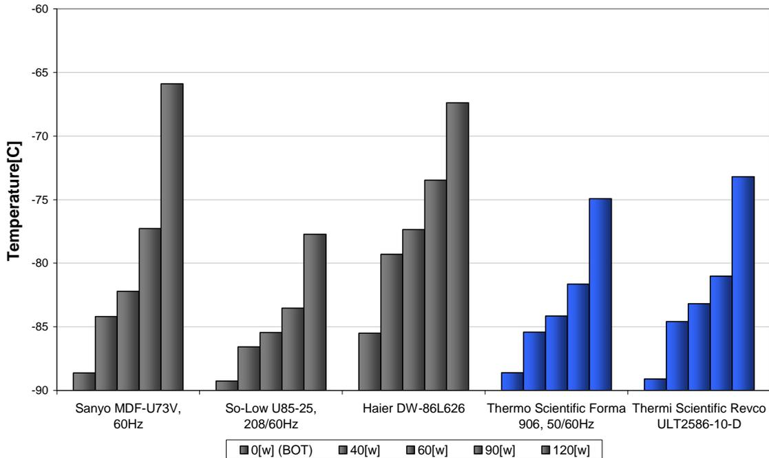
Figure 3 demonstrates the time it takes for an empty ULT to warm from -80°C to -50°C during a simulated power outage and is based on an average cabinet temperature. During prolonged power outages, freezers will warm over time. The length of time to warm is based on the cabinet's insulation properties and the door seal. Fully-loaded or partially loaded freezers will warm more slowly than an empty freezer. However, this test provides a baseline for this performance.
